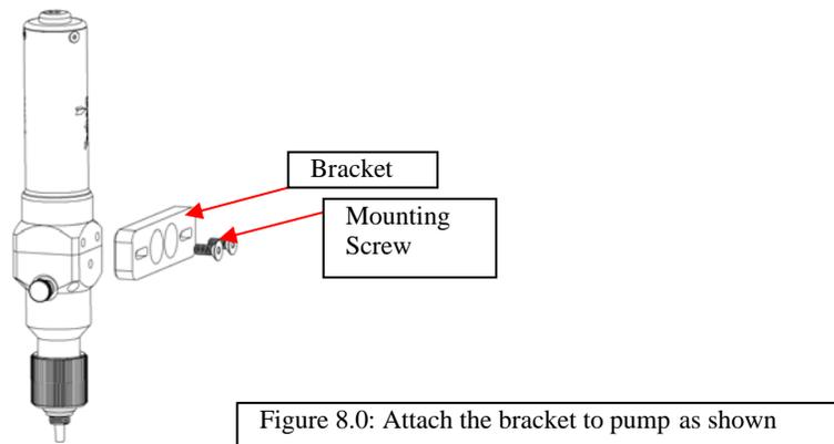
Figure 8.0: Attach the bracket to pump as shown
