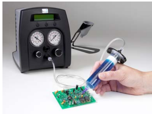
Figure 1. A precision dispenser that features a digital timer to dispense small dot of fluid accurately from a syringe
